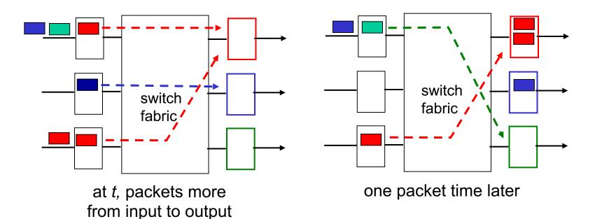
buffering when arrival rate via switch exceeds output line speed
